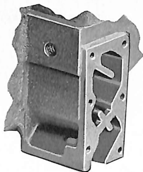
Fig. 2. View of the Crank Case Vent with Cover Removed showing Baffles in the Air Passage
